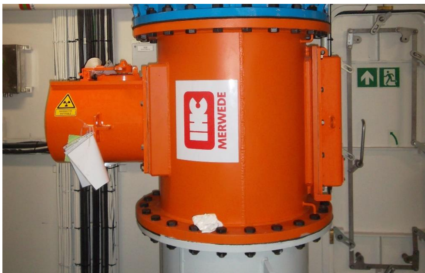
Figure 1. The RadioActive (RA) density meter, commonly used in the dredging industry
