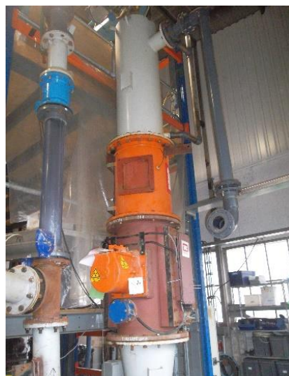
Figure 6. The small scale test circuit with two stacked RF measurement pipes (orange and brown) are visible. The transparent high flow water pipe, used to agitate the flow in the column, is visible to the left
