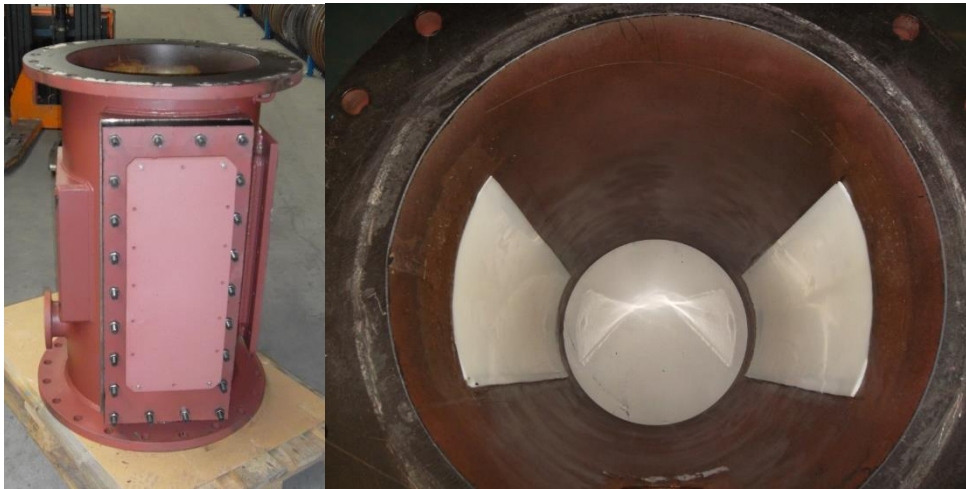
Figure 4. The non-radioactive RF density measurement pipe. A rectangular flange lid hiding the antenna (left), and the irathane flush-mounted dielectric windows on the inside of the pipe are visible (right)
