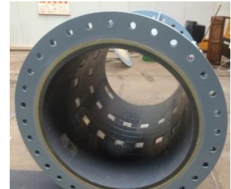
Figure 5 Tomography sensor with ceramic liner and duplex electrodes
