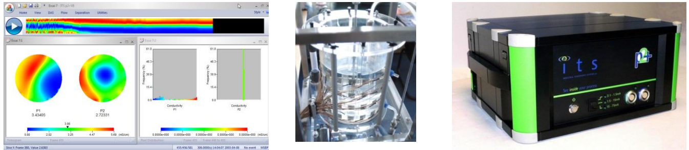
Figure 1 Tomography system configuration; software, sensors, instrument
